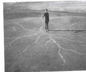
Photograph showing evidence of electrical breakdowns across the Earth's surface from the current of natural lightning injected into a grounding electrode. In this case the pole on a golf course green. Courtesy of E. Philip K. Sides.
