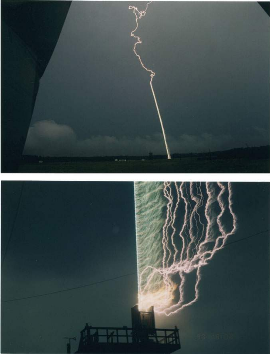
Fig. 19 Photographs of lightning flashes triggered using the rocket-and-wire technique at Camp Blanding, Florida. Top—a distant view of a strike to the test airport runway; bottom—a close-up view of a strike to the test power system
