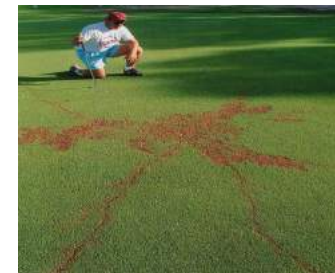
Photograph showing evidence of electrical breakdowns across the Earth's surface from the current of natural lightning injected into a grounding electrode. In this case the pole on a golf course green. Courtesy of E. Philip K. Sides.
