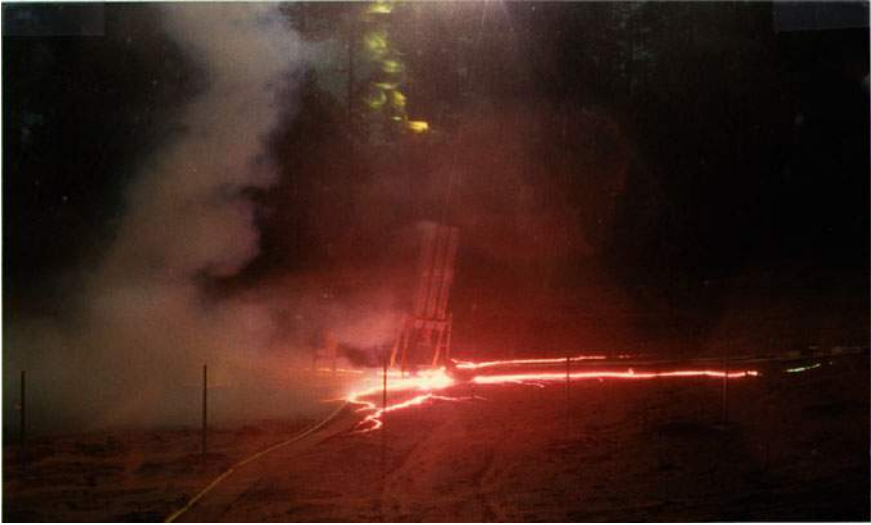
Fig. 20 Photograph of surface arcing associated with the second stroke (current peak of 30 kA) of flash 9312 triggered at Fort McClellan, Alabama. Lightning channel is outside the field of view. One of the surface arcs approached the right edge of the photograph, a distance of 10 m from the rocket launcher. Adapted from Fisher et al. [8]
