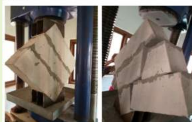
Lab test of AAC prism in diagonal compression (Shear test)
