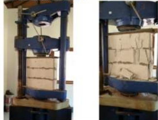
Lab test of the AAC Prism in compression.
